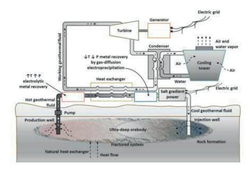
Figure 3 Concept of a combined heat, power and metal extraction geothermal plant (based on horizon 2020 project CHPM2030: https://www.chpm2030.eu/introduction/).
