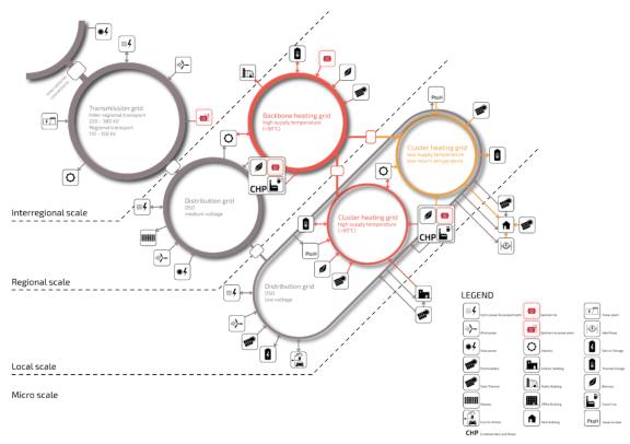
Figure 2 Hybrid energy infrastructure composed of interconnected energy networks based on renewable energy sources (courtesy of DNV GL, based on: NoordhoffUitgevers B.V., 2012) – extended version of VISION Fig. 10, including synthetic fuel and gas.
