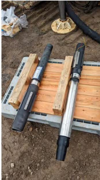
DTH hammer and Tool joint for Real time, fast data connection / transfer
