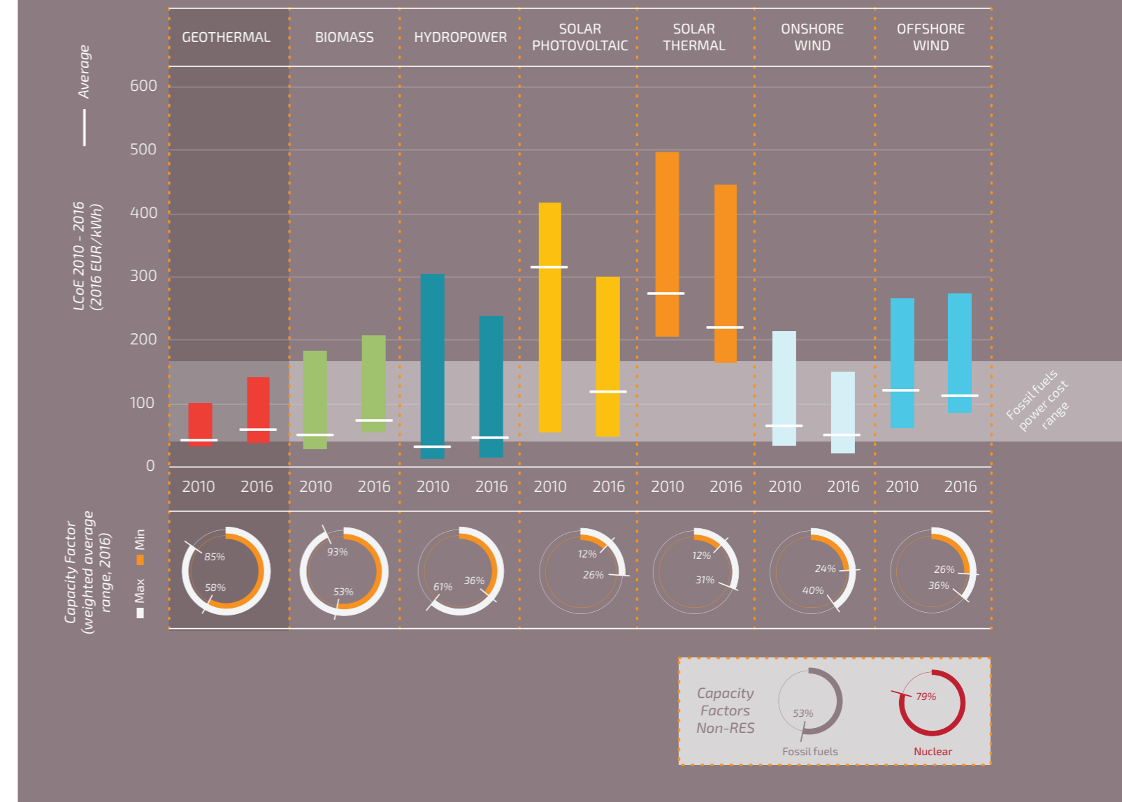
● FIGURE 3 Since geothermal energy is constantly provided, the Capacity Factor (i.e. actually produced energy with respect to the full capacity) is much higher than for other renewable energy sources (sources: Renewables 2017 Global Status Report, REN21; EUROSTAT), resulting in a total cost (LCoE) comparable or lower than for other energy sources (source: IRENA, 2017)
